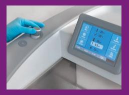
NX70 cryostats feature motorized sectioning for ease of use and to reduce the need for repetitive motions
